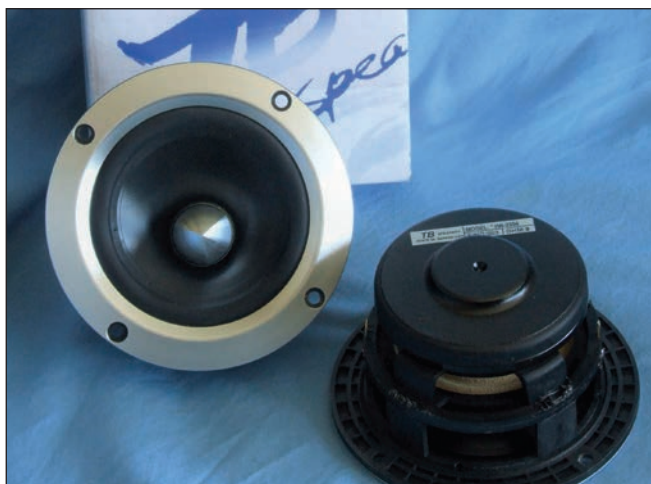
Photo 1: The first thing you should notice about TB Speaker's W4-2356 is that the voice coil is not centered in the 4" injection molded polypropylene cone, but offset by about 0.5".
